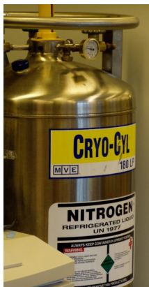
A tank of liquid nitrogen, used to supply a cryogenic freezer (for storing laboratory samples at a temperature of about -150^{\circ}\text{C} ).
